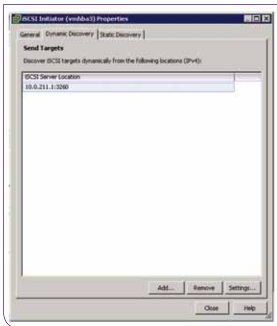
Figure 3. Automatic discovery of iSCSI targets
