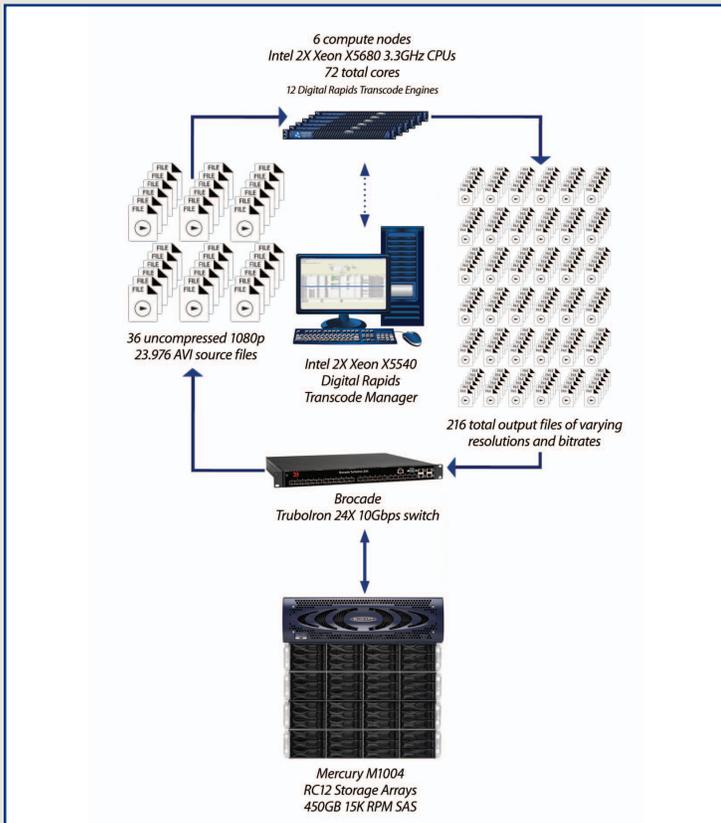
The transcoding workload consisted of 36 uncompressed 1080p23.976 AVI source files, each of which was transcoded to six different resolutions/bitrates using H.264 video and AAC audio compression in an MP4 container: one 1920p, three 720p at varying bit rates, and two 480p at varying bit rates. The encoding parameters used were the actual profiles used by a major studio to create premium deliverables for audience distribution.
