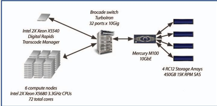
Six systems based on Intel 2X Xeon X5680 processor series, multi-threaded, multi-core 3.3GHz CPUs with 24GB RAM were used to host 12 Digital Rapids Transcode Engines, and a single system based on an Intel 2X 5540 processor series 2.5GHz CPU with 24GB RAM ran Digital Rapids Transcode Manager software.
