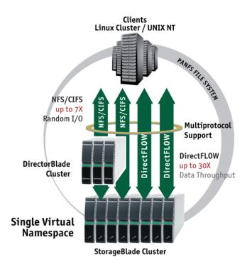
is completely transparent to both the user and application. Furthermore, when new capacity is introduced, PanFS automatically load-balances the system by targeting new data writes to the new capacity and migrating as much of the existing data as required. The solution therefore always maintains a balanced performance.
