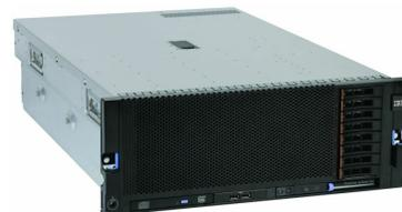
The System x3850 X5 was set up running Windows Server 2008 R2 and SQL Server 2008. The server had two dual-port Emulex OneConnect OCe10102-F 10Gbps FCoE adapters running the standard Emulex driver for Windows Server 2008 R2 x64 (driver version 2.30.016). The Emulex OneCommand™ Manager application was used to monitor FCoE connectivity on the server.
