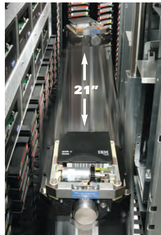
In just 21" of horizontal travel the XLS robot can access over 3,200 tapes.
