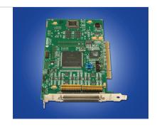
Performance Technologies' PCI334A Intelligent Synchronous WAN Communications Adapter provides four high-performance synchronous/serial channels for WAN connectivity. The adapter is ideally suited for use within radar networks, frame relay access devices, high-speed modems, or other high-speed communication devices.
